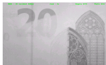
Fragment of the examined banknote in infrared incident light (830 nm). 2x magnification on the monitor
