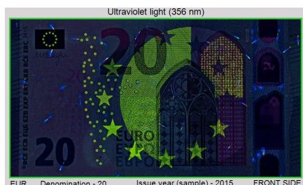
Comparison of the examined banknote in ultraviolet light (365 nm) with the reference banknote from the database
