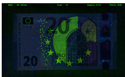
Comparison of the examined banknote in ultraviolet light (365 nm) with the reference banknote from the database
